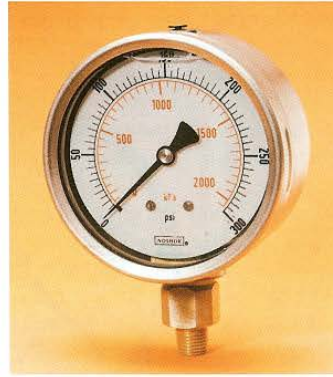
25.901 2 1/2 INCH STAINLESS STEEL CASE GLYCERINE FILLED 1/4" NPT BOTTOM CONNECTION
