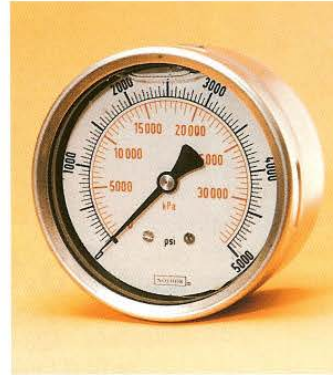
25.911 2 1/2 INCH STAINLESS STEEL CASE GLYCERINE FILLED 1/4" NPT CENTER BACK CONNECTION
